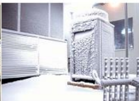
Environment simulation lab from -40°C -55°C & snowfall simulation
